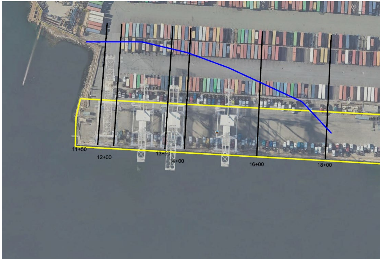
Figure 20: Proposed Bulkhead Wall Location at Various Cross-Sections
